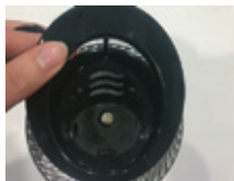
Retirez la vis cruciforme
