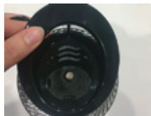
Retirez la vis cruciforme
