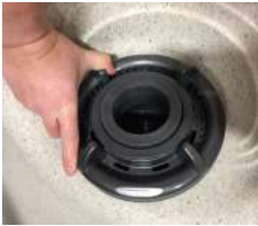
Twist Lock Ring Counter-clockwise to Remove Floater
