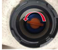
Turn Filters Counter-clockwise to Remove
