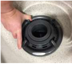
Twist Lock Ring Counter-clockwise to Remove Floater
