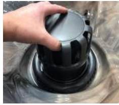
Pull Up to Remove Floater Assembly
