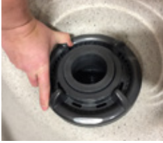
Twist Lock Ring Counter-clockwise to Remove Floater
