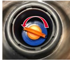
Turn Filters Counter-clockwise to Remove
