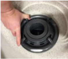
Twist Lock Ring Counter-clockwise to Remove Floater
