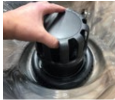
Pull Up to Remove Floater Assembly
