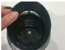
Retirez la vis cruciforme
