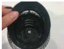
Retirez la vis cruciforme
