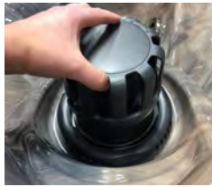
Pull Up to Remove Floater Assembly
