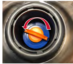
Turn Filters Counter-clockwise to Remove
