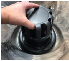
Pull Up to Remove Floater Assembly
