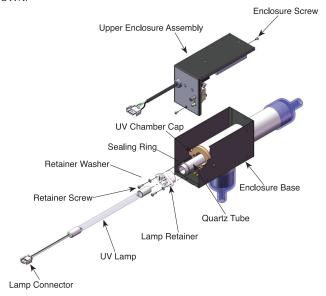
Figure 2: Spa Solar Eclipse Exploded View
