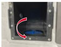
Turn Filter Counter-clockwise to Remove
