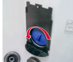
Turn Filters Counter-clockwise to Remove
