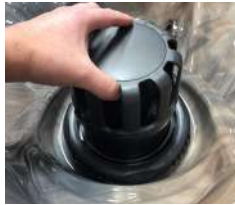
Pull Up to Remove Floater Assembly
