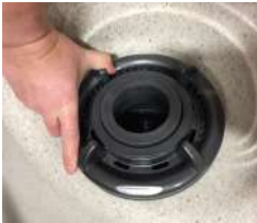
Twist Lock Ring Counter-clockwise to Remove Floater
