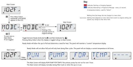
If the primary pump has been off for an hour or more, when any function button, EXCEPT Light, is pressed on the panel, the pump used in conjunction with the heater will run so that temperature can be sensed and displayed.
