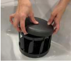
Remove Top Cap by Gently Lifting
