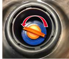
Turn Filters Counter-clockwise to Remove
