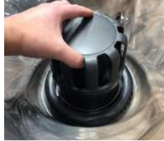
Pull Up to Remove Floater Assembly
