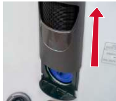
Slide Faceplate Up to Remove
