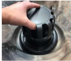
Pull Up to Remove Floater Assembly
