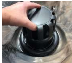
Pull Up to Remove Floater Assembly
