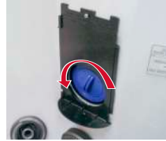
Turn Filters Counter-clockwise to Remove
