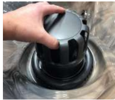
Pull Up to Remove Floater Assembly
