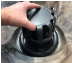
Pull Up to Remove Floater Assembly
