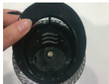
Retirez la vis cruciforme
