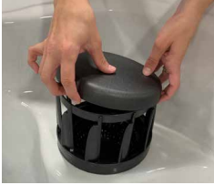
Remove Top Cap by Gently Lifting
