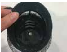
Retirez la vis cruciforme
