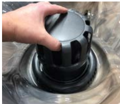
Pull Up to Remove Floater Assembly
