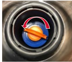
Turn Filters Counter-clockwise to Remove
