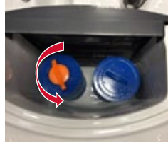
Turn Filters Counter-clockwise to Remove
