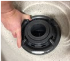
Twist Lock Ring Counter-clockwise to Remove Floater
