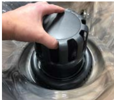
Pull Up to Remove Floater Assembly
