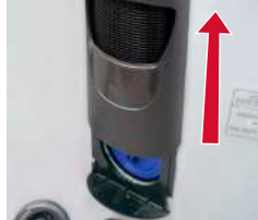
Slide Faceplate Up to Remove
