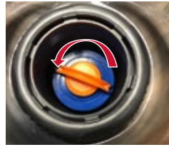
Turn Filters Counter-clockwise to Remove
