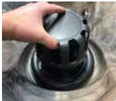
Pull Up to Remove Floater Assembly
